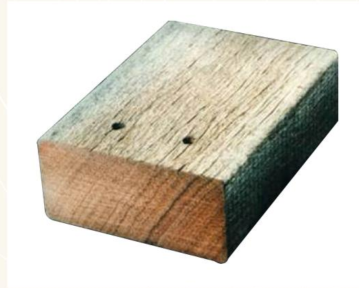
Ipe decking after 25 years on the Atlantic City Boardwalk
